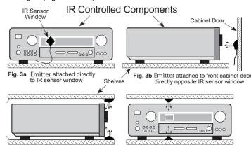
Fig. 3c & d Emitter attached to shelf directly below or above IR sensor window
